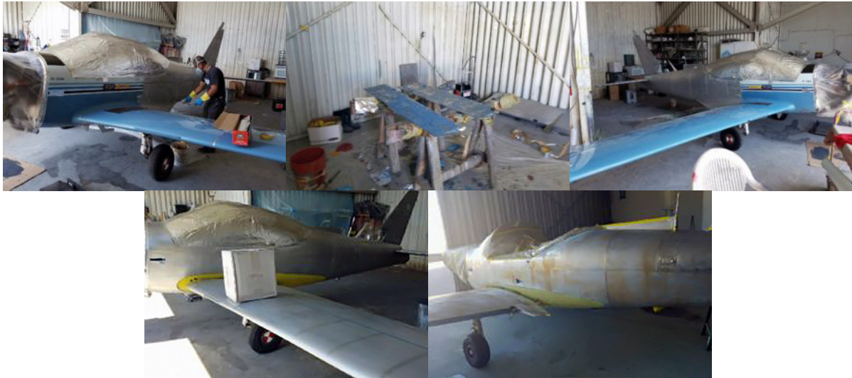
The paint is stripped and the aircraft coated with anti-corrosion product (© Sebastien Dominé)
